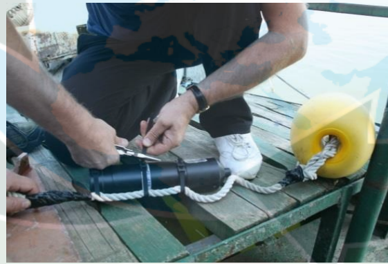
Figure 6: Reception station installed on the rayon wire
